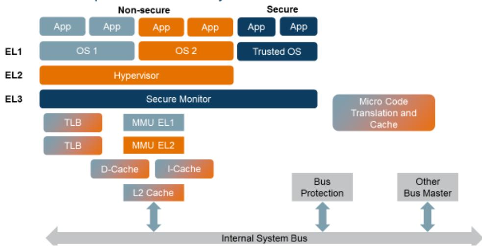
This architecture has three privileged exception levels. Exception level 1 is owned by the operating system and allows to configure the first level Memory Management Unit (MMU).
