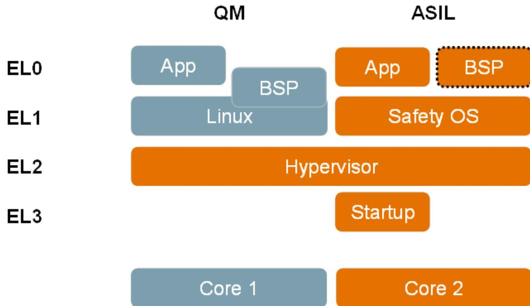
In case the safety OS only uses generic functions of the ARMv8 architecture it may be even feasible to qualify as stripped down Linux to perform the functionality of the safety OS.
