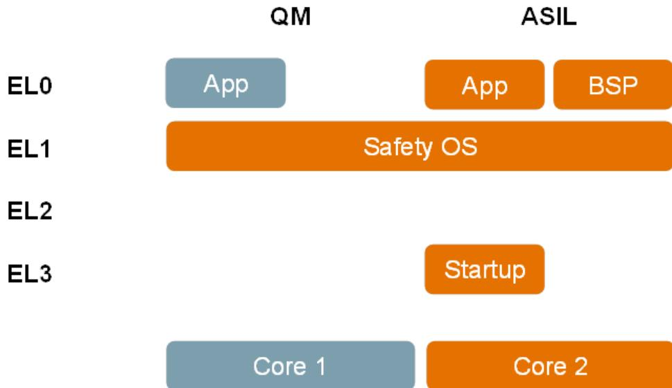
The simplest setup at first glance is to have a safety operating system, which is safety certified and executes QM and ASIL functions. Ideally they are dedicated to different cores so that the Bus Protection can discriminate between them. Performing a fine grained prevention of wrong map access on OS level is possible, but tedious and the QM applications would have to be modified. Most likely the BSP has to be safety certified as well.
