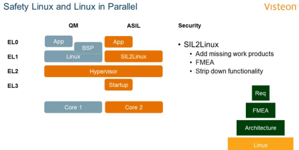
This and even more is done by the SIL2Linux project. The safety relevant work products have to be provided to be able to qualify Linux. The change rate and code size are problems for this approach. So it
