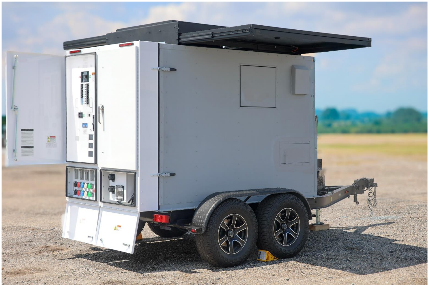
The mobile battery energy storage system known as Green Grid 90 kWh mobile battery energy storage system (MBESS) can generate power via solar panels on its roof – or it can be plugged in and store energy for later.
