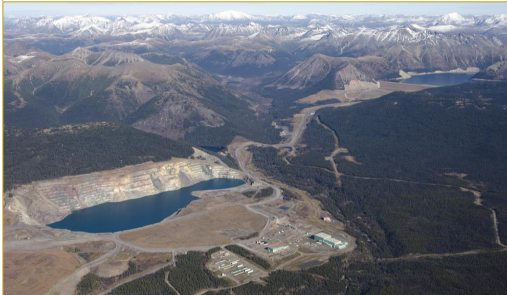
Figure 6: Kemess tailings storage using the previously mined pit as well as an existing tailings facility, which is capable of expansion.
