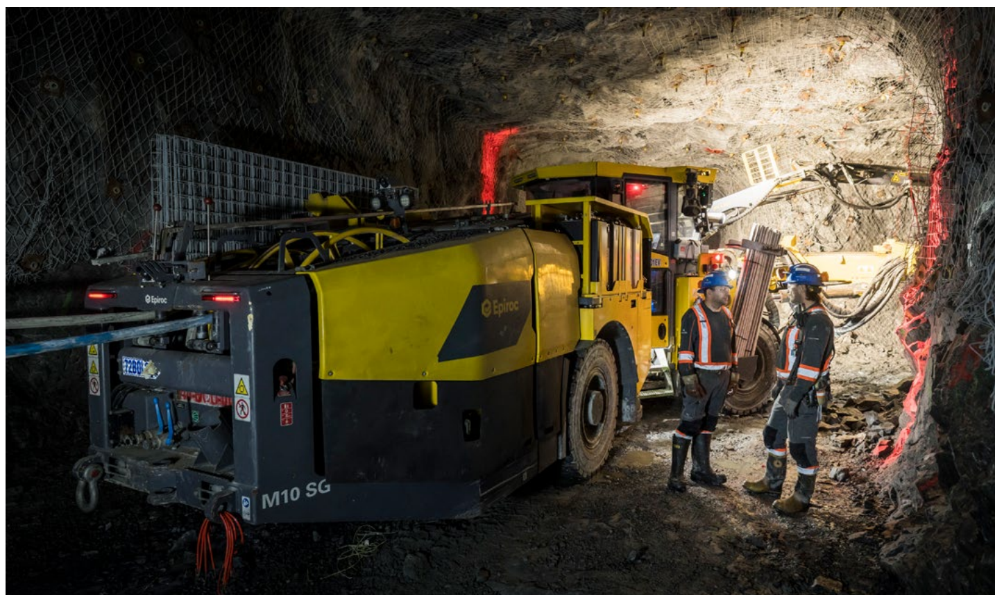
Battery electric bolter at Odyssey (Quebec, Canada).
