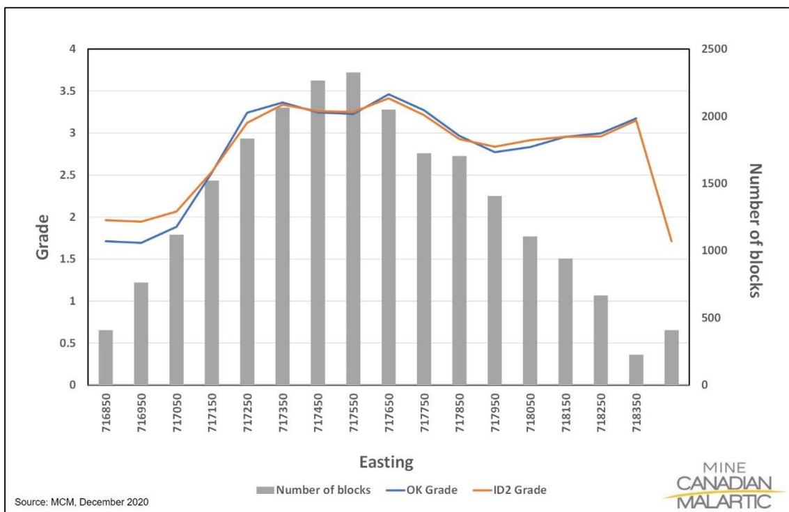
Figure 14.13 – Swath plot in easting of the East Gouldie block model, comparing OK and ID2 block model grade values
