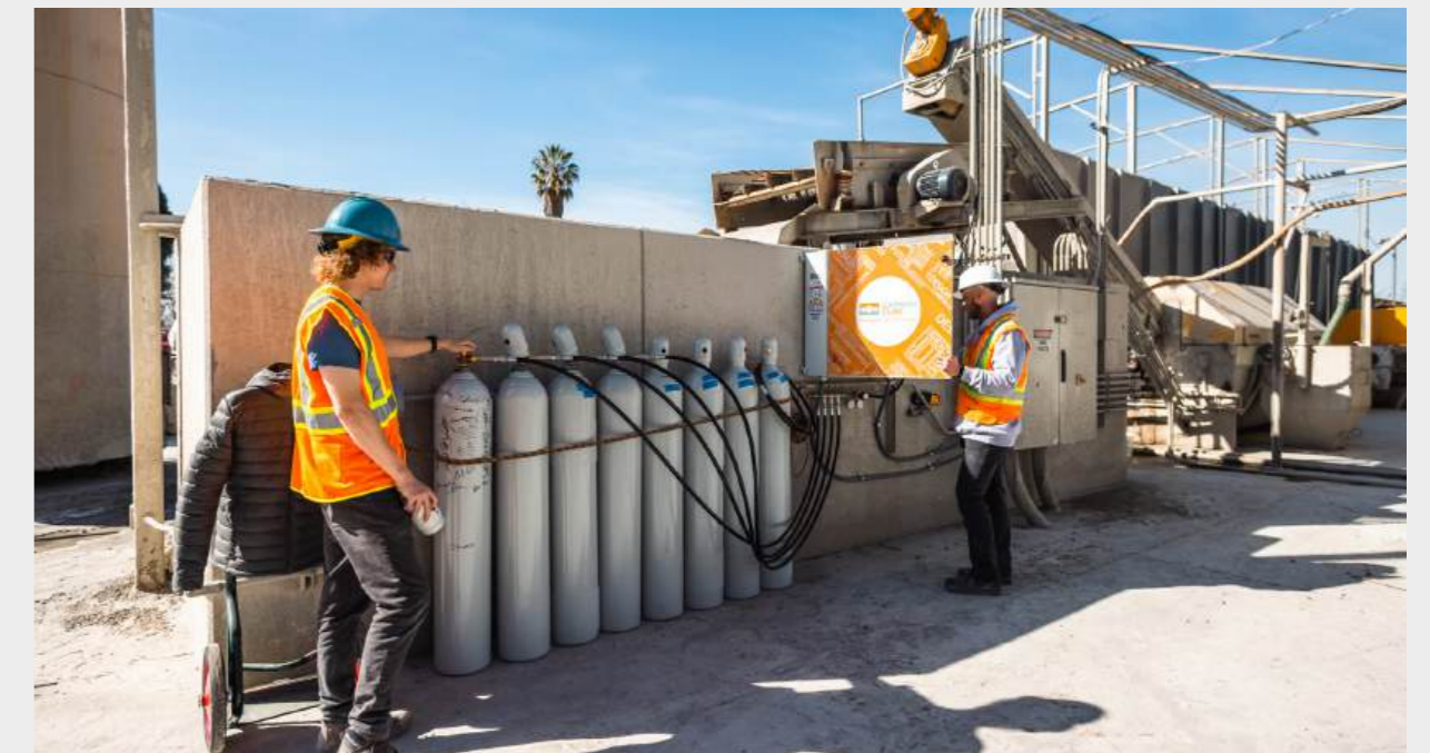
CarbonCure technology injects captured CO 2 into fresh concrete to permanently mineralise it, reducing carbon footprint without sacrificing strength. Image courtesy of CarbonCure Technologies.
